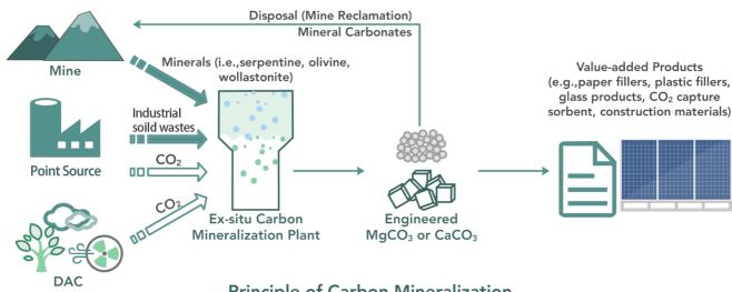
Principle of Carbon Mineralization
